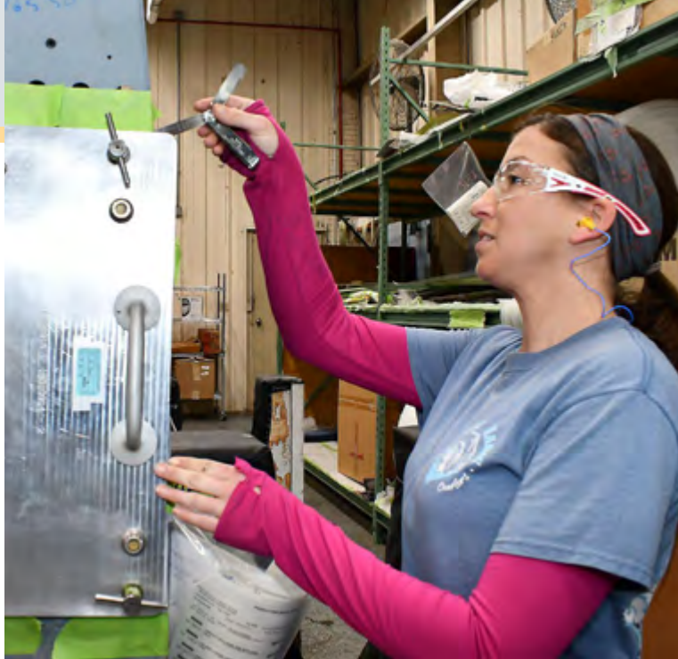
Shevaun Jones, a sheet metal worker in the H-53 Aircraft Components Shop at Fleet Readiness Center East (FRCE), uses a feeler gauge to check for excessive gaps on the mount feet of an H-53 spar fitting.
