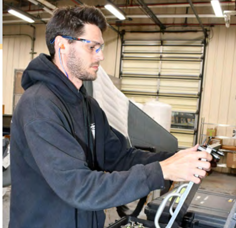
Michael Wells, a sheet metal worker in the H-53 Aircraft Components Shop at Fleet Readiness Center East (FRCE), prepares a plate used to check an H-53 spar fitting's mount feet for excessive gaps.
