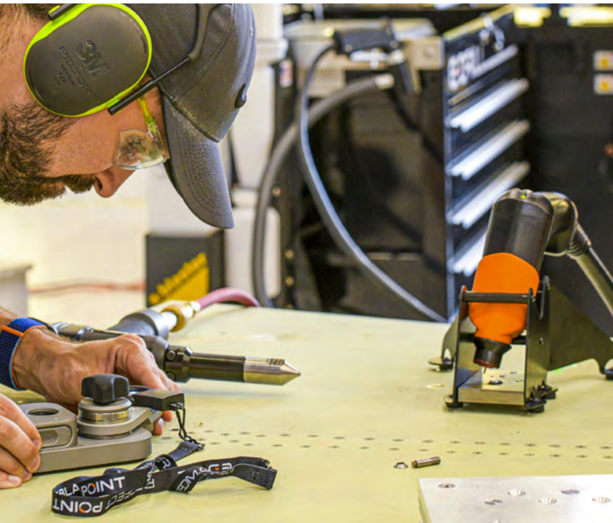
Charles Newton, a senior materials engineer with Fleet Readiness Center Southeast (FRCSE), uses an E-Drill system to remove fasteners on an F-5 Tiger II horizontal stabilizer. FRCSE’s F-5 Production Line is the first to implement the E-Drill within the NAVAIR enterprise. The device will significantly reduce the time it takes to remove the thousands of rivets typically replaced during in-depth depot-level maintenance.
