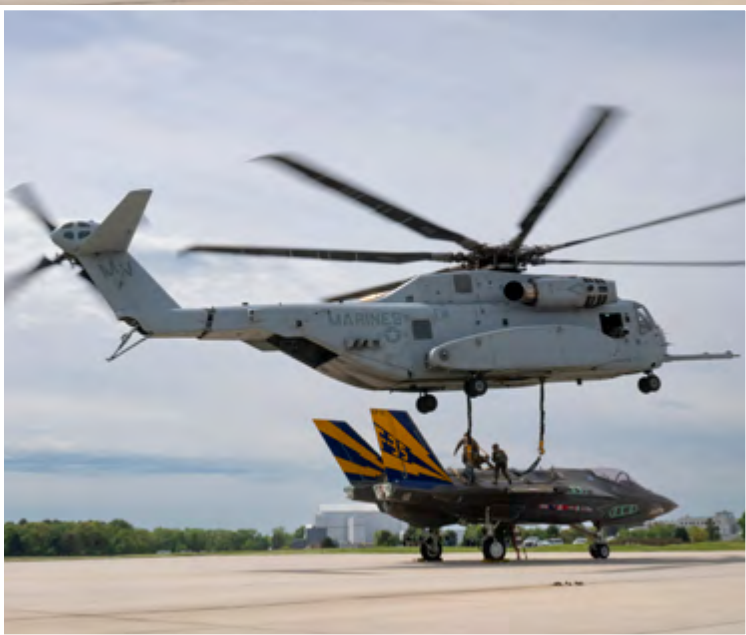
Marine Corps members of the Helicopter Support Team from Combat Logistics Battalion 26 attach a non-flying F-35C airframe from the NAS Patuxent River F-35 Integrated Test Force to a sling beneath a hovering CH-53K, operated by Marine pilots from VMX-1, at NAS Patuxent River April 24.
