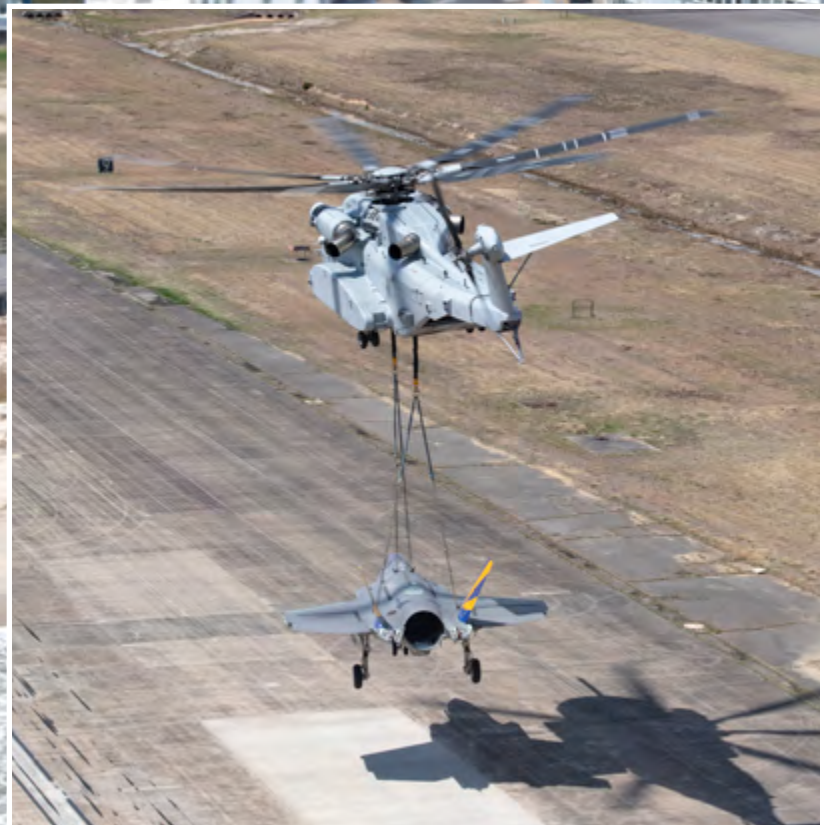
Marine Corps pilots from VMX-1 flying a CH-53K helicopter lower a non-flying F-35C airframe from the NAS Patuxent River F-35 Integrated Test Force onto the runway at Joint Base McGuire-Dix-Lakehurst, New Jersey, on April, 24, after transporting the F-35C airframe from NAS Patuxent River, Maryland. The transportation of the airframe will enable future testing at Lakehurst of emergency recovery systems.
