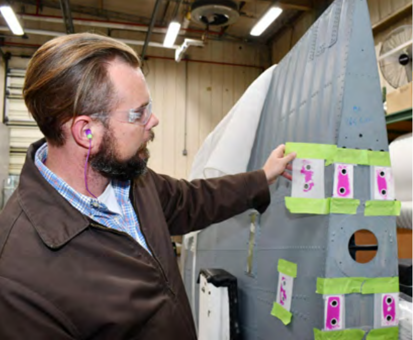
Jason Gaskill, an H-53 airframe production support engineer with the Maintenance, Repair and Overhaul Engineering Production Line Support Division at Fleet Readiness Center East (FRCE), examines successive rounds of impressions left by pressure-sensitive film while checking contact surfaces on the mount feet of an H-53 spar fitting.
