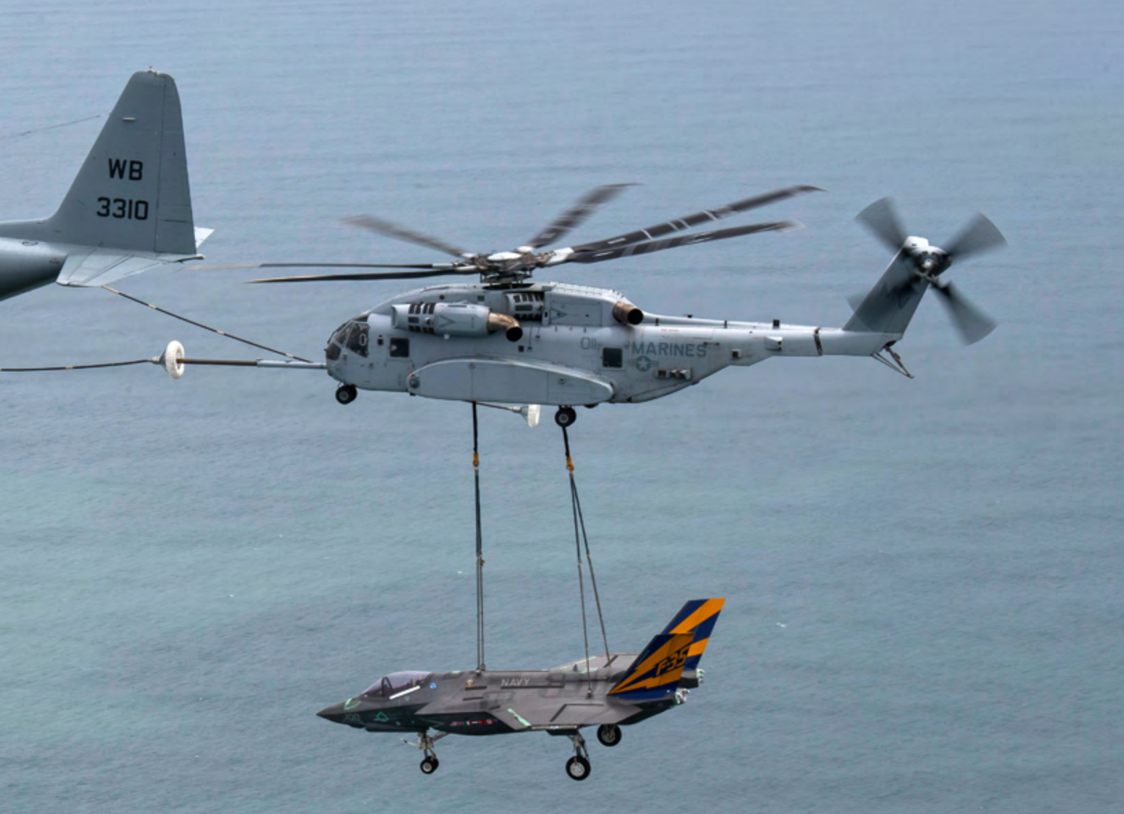
Marines from VMX-1 pilot a CH-53K helicopter over the Chesapeake Bay in Maryland, conducting aerial refueling from a C-130T operated by Navy's VX-20 while carrying a non-flying F-35C test airframe from the NAS Patuxent River F-35 Integrated Test Force on April 23. The flight was conducted in preparation for the aerial transport of the non-flying F-35C airframe from NAS Patuxent River, Maryland, to Joint Base McGuire-Dix-Lakehurst, New Jersey, the following day.
