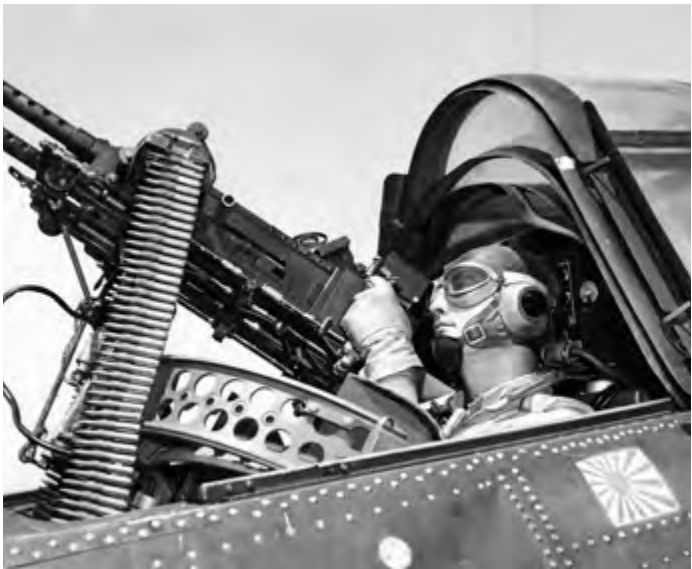
The rear-seat gunner of an SBD dive bomber could have a single, or in this case, two .30 caliber machine guns (later in the war) to defend his aircraft and others in his formation. Note the single Japanese kill flag below him. Coordination and dependability were the hallmarks of these two-man crews.
